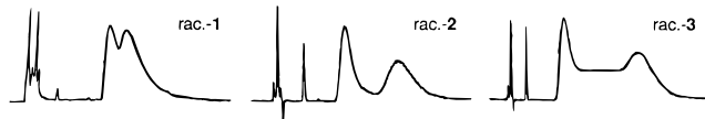
Figure 1. Chromatographic separation of racemic telluroxides 1 , 2 , and 3 on an optically active column (AS) by means of HPLC.
